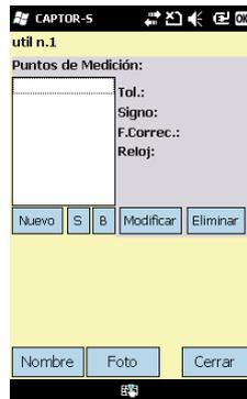
4. To make the identification of the gauge easier, we recommend you to take a general picture of the gauge by clicking on *“Photo”*. Define the measurement features: number of points (add, modify or delete), tolerances, correction factor (if necessary), type of dial indicator.
