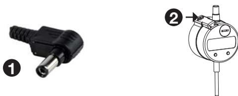
2. Charging the dial indicator: connect the 2.1 port(1) To the dial indicator connector (2). Plug the charger in. It will take 3 hours to charge it completely. The dial indicator does not have any level of battery display. If you see that your device does not emit any signal, it may be due to a low battery level.
