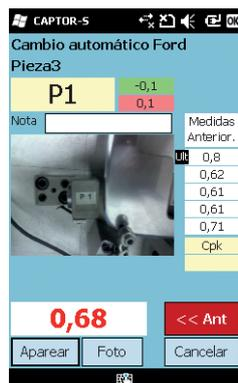
5. Click on the button (4). The measured value will be displayed on the screen, as well as whether the value is within our out of tolerance. Then, Captor will pass automatically to point 2.
