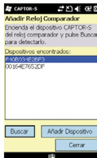
3. Select your dial indicator and click on “Add Dial Indicator”. The PDA may detect other devices close to it, such as Bluetooth mobile phones. To identify your CAPTOR-S, you will have to check the ID number displayed on the sticker on the back part of the device. You can check if your CAPTOR-S works properly by using the PDA test function. To use this function, turn the dial indicator and the Bluetooth unit on, and press the “Test” button on the PDA screen.
