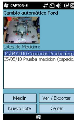
2. In each of the gauges folders, you can define measurement groups, that is, a group of measured parts with a common feature (month of measurement, first injection, etc.). To add new measurements in an existing group, select the corresponding group and click on “Measure”.
