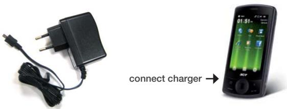
b. By electric plug: connect the Micro USB port to the PDA and plug in the charger. A red LED will turn on on the PDA upper right side.
